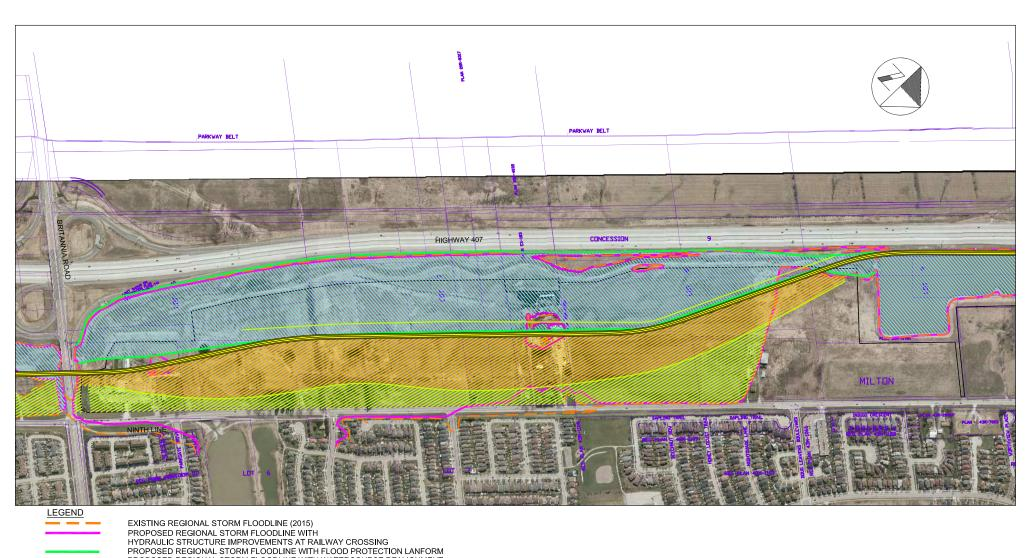
PROPOSED REGIONAL STORM FLOODLINE WITH WATERCOURSE REALIGNMENT EXISTING RIGHT OF WAY PROPOSED TRANSITWAY REGIONAL STORM FLOODPLAIN REMOVED - POTENTIAL DEVELOPABLE AREA (RESTRICTED) REGIONAL STORM FLOODPLAIN REMOVED - POTENTIAL DEVELOPABLE AREA (UNRESTRICTED)
