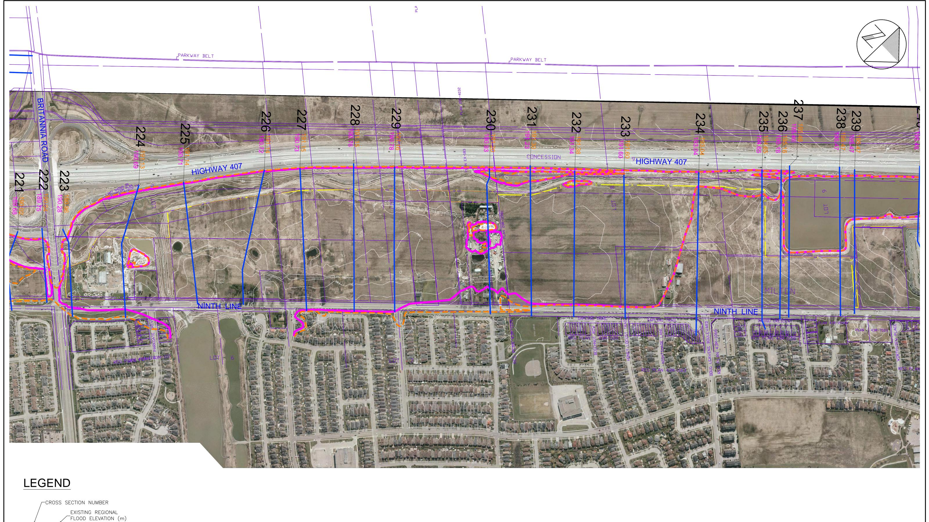
HEC-RAS CROSS SECTION LOCATION PROPOSED REGIONAL FLOOD ELEVATION (m) EXISTING REGIONAL FLOODLINE (2015) PROPOSED REGIONAL FLOODLINE WITH HYDRAULIC STRUCTURE IMPROVEMENTS AT CNR
