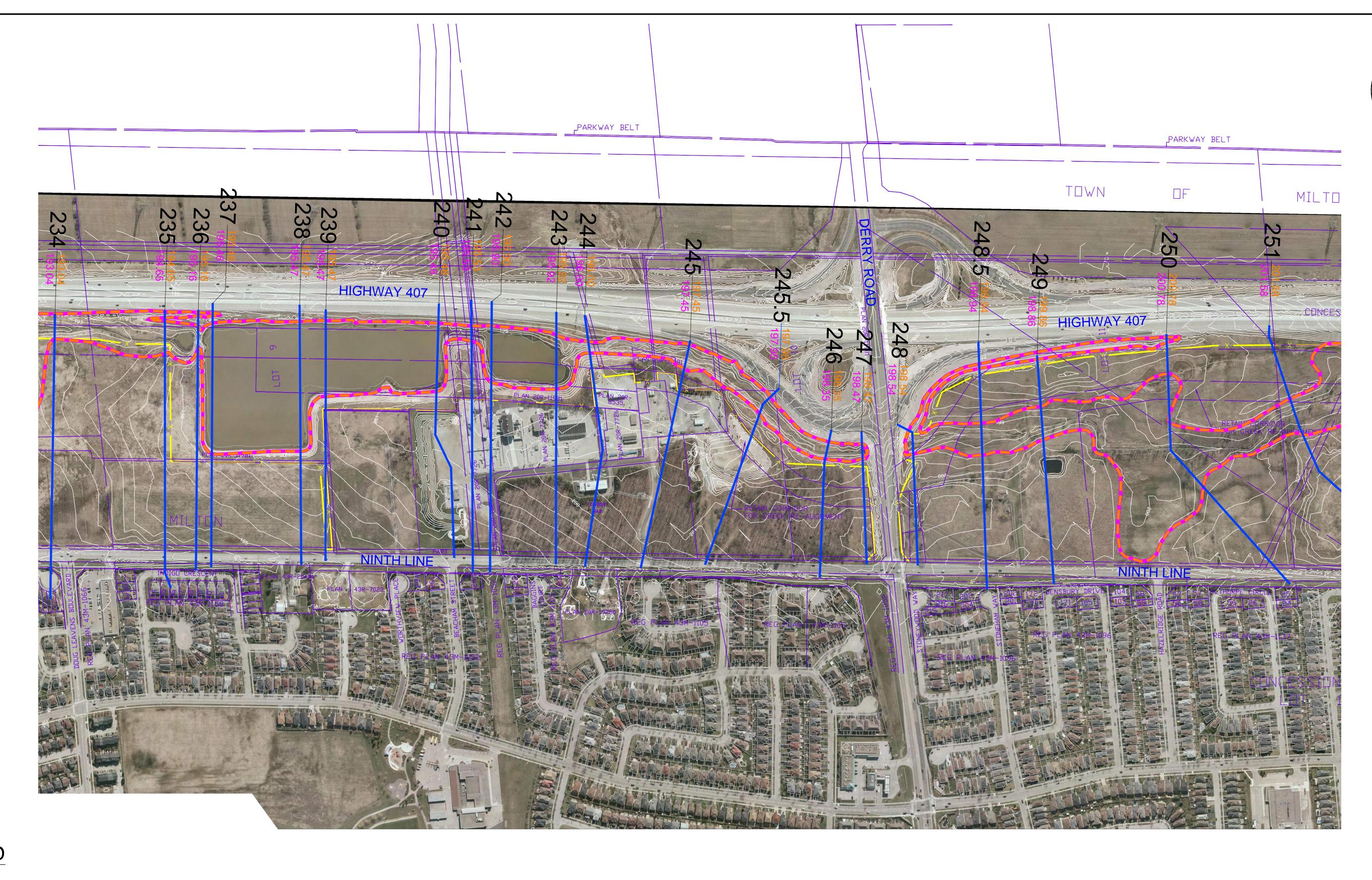
CROSS SECTION NUMBER EXISTING REGIONAL FLOOD ELEVATION (m) HEC-RAS CROSS SECTION LOCATION PROPOSED REGIONAL FLOOD ELEVATION (m) EXISTING REGIONAL FLOODLINE (2015) PROPOSED REGIONAL FLOODLINE WITH HYDRAULIC STRUCTURE IMPROVEMENTS AT CNR EXISTING HIGHWAY 407 FENCELINE
