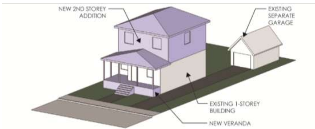
Figure 21: Example of new 2nd-storey addition with veranda on a 1-storey building on a contributing property
