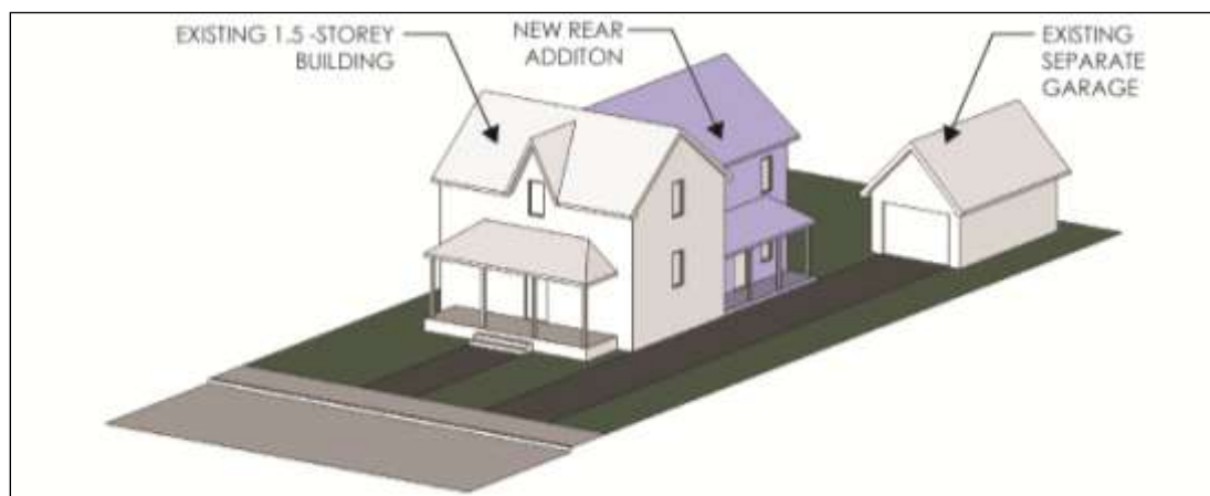
Figure 18: Example of new rear 1.5-storey addition for building on a contributing property
