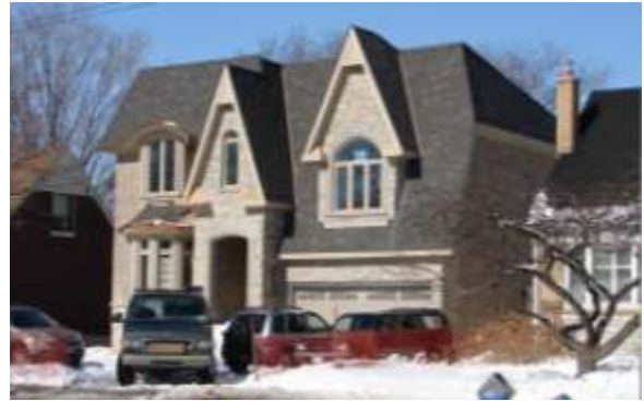
Figure 32: An example of an unsuitable contemporary house. Faux stone cladding, and several different types of faux historic gables and roof shapes are discouraged.
