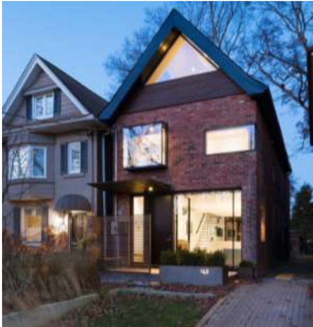
Figure 23: An example of a suitable contemporary house alteration on a contributing property. New is differentiated from old, while the original roofline is maintained. The garage is separate and located in the rear. Credit: Johnson Chu, architect / Brenda Liu, photographer.
