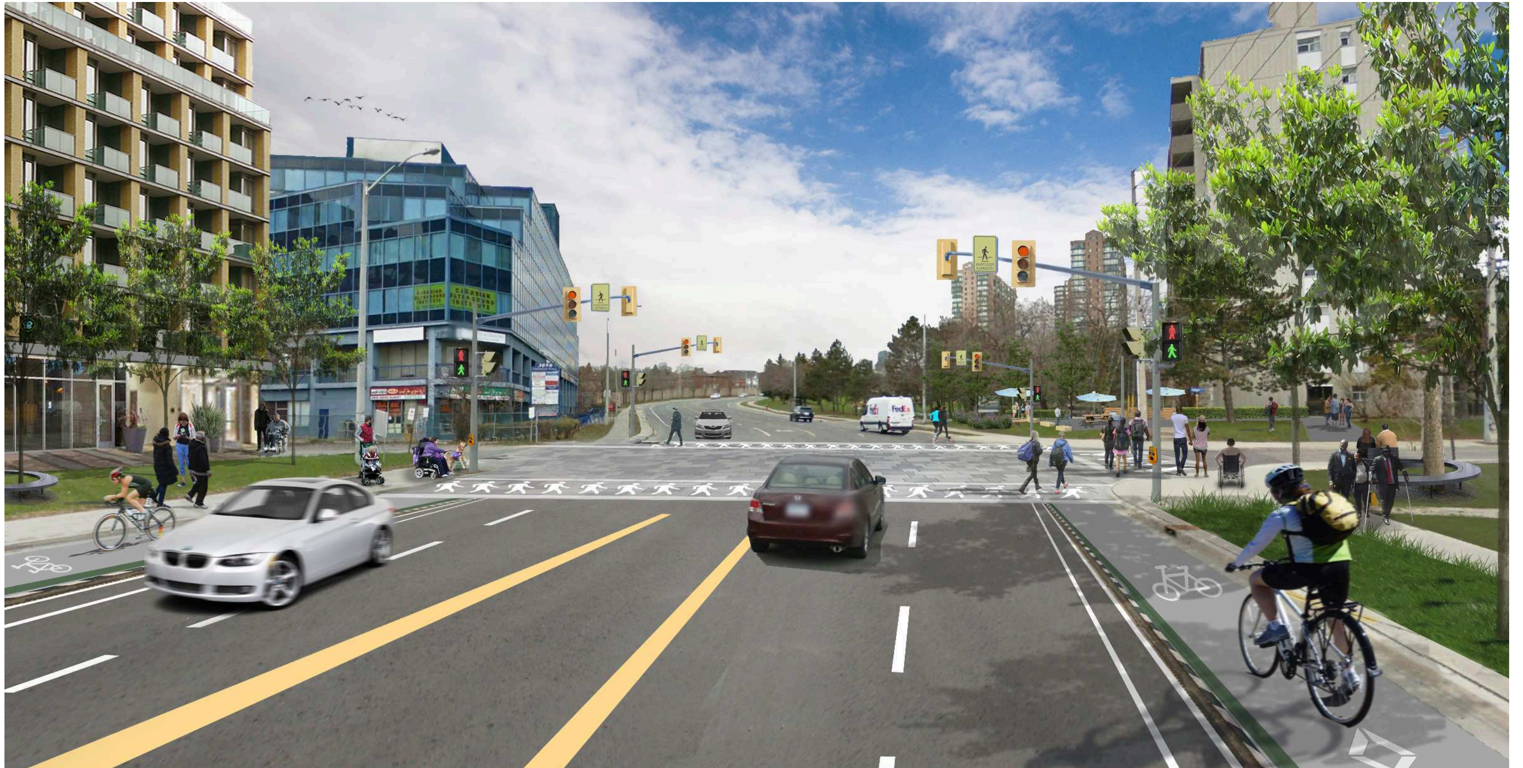
FIGURE 2.7 - Confederation Pkwy and Agnes St. (after): Pedestrian safety improvements can be achieved through the use of distinct material treatments, cross walks and signals that indicate safe pedestrian crossing areas and separated bicycle lanes.
