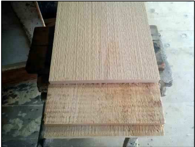
1 X 12 (NOMINAL) ROUGH SAWN KILN DRIED PINE BOARDS SOURCE: HOFFMEYERS MILL, 189 HURON RD., SEBRINGVILLE ON
