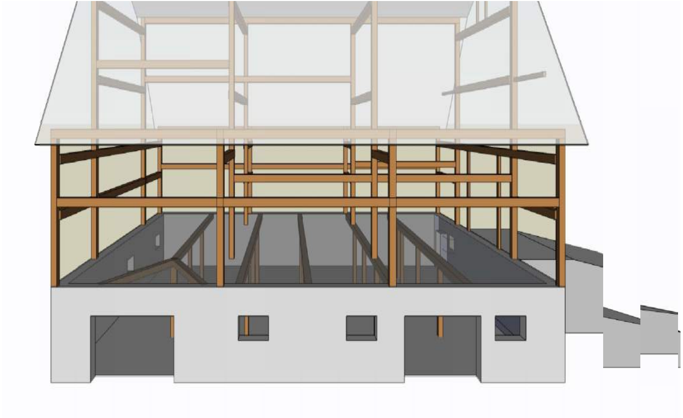
Figure 5.31 Conover Barn. Perspective Elevation showing structural elements.
