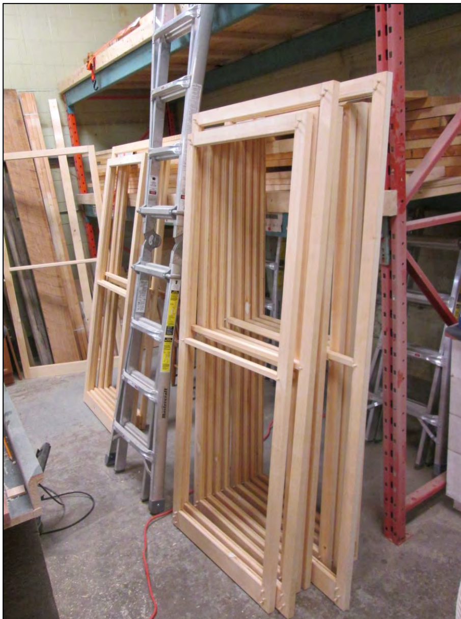
Storm windows glued, assembled and pegged
