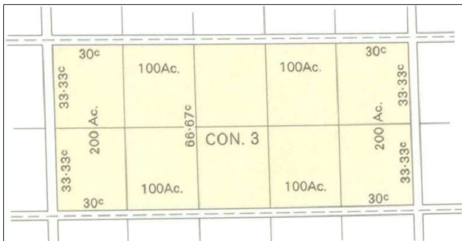
Plate 2: Double-front survey system (Dean 1969)
