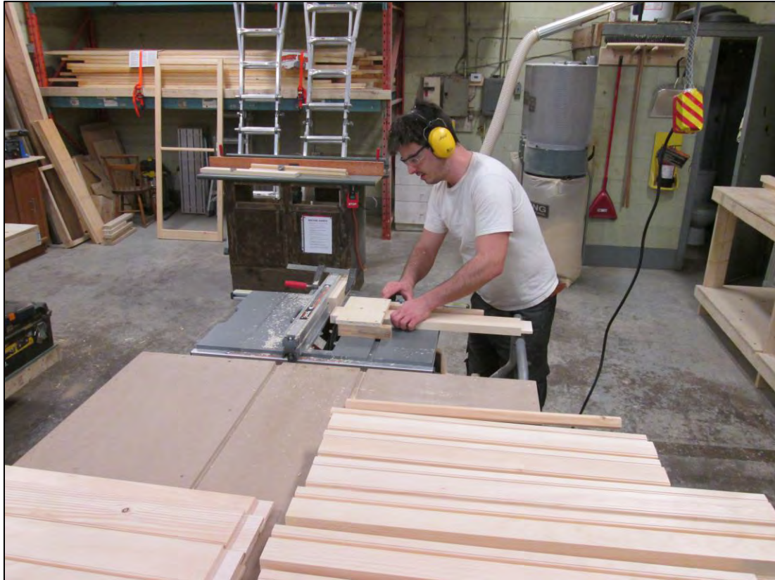
Cutting the tenons with the dado set
