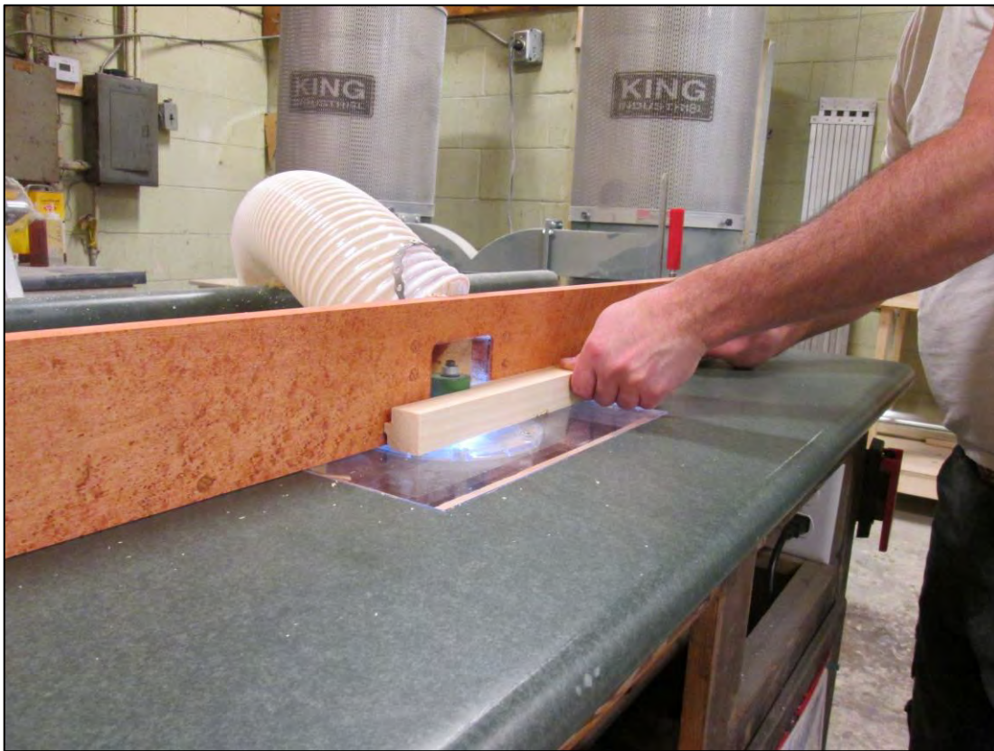
Running the rebate and Roman ogee on the router
