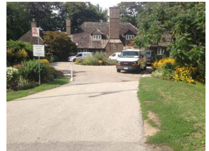
② ENTRANCE DRIVE CIRCLE TO BE RE-PAVED WITH CHIPSET ASPHALT AND STONE EDGE
