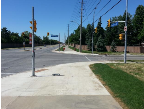
Figure 7: At the Tours Road intersection, cyclists legally must dismount to cross. However in practice, many ride through. The trail leads into a full curb, which is potentially dangerous for cyclists who may expect a ramp. Cyclists may use the curb cut to the left, which is very close to turning traffic, or the one to the right, in which they may lose sight of traffic by turning away from the roadway, and conflict with pedestrians in the narrow sidewalk space.
