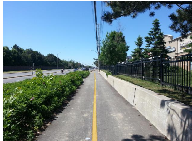
Figure 6: Adding a solid centreline in narrow stretches encourages users to walk and ride along the edges of the trail, instead of the middle. This makes passing easier, and leads to less conflicts between users travelling at different speeds.
