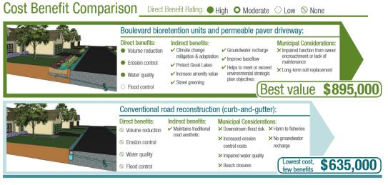
LID usage leads to considerable construction, operation and maintenance savings. The Lakeview and Elm Drive demonstration projects, both constructed by the City of Mississauga and the CVC, were 18% and 10% cheaper to build that
