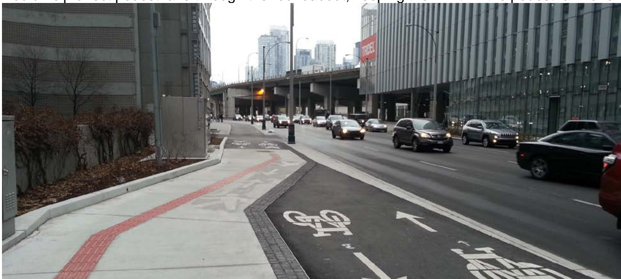
Image: Directional tactile walking surface indicators (red line) directing pedestrians to sidewalk from shared space, City of Toronto
