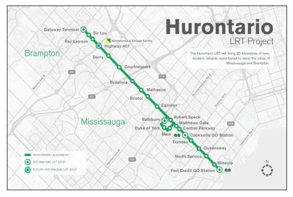
New, modern light rail vehicles will travel in a dedicated right-of-way and serve 22 stops serving 2 urban growth centres, 4 mobility hubs, and connections to GO Transit's Milton and Lakeshore West rail lines, MiWay, Brampton Transit, and the Mississauga Transitway. The LRT will provide up to 5 minute service frequencies both ways during peak periods. Light Rail Vehicles will operate in a segregated guideway ensuring reliable and convenient service to passengers.
