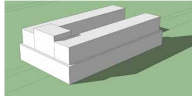
Diagram 19A: Two Slab Through Unit Massing
