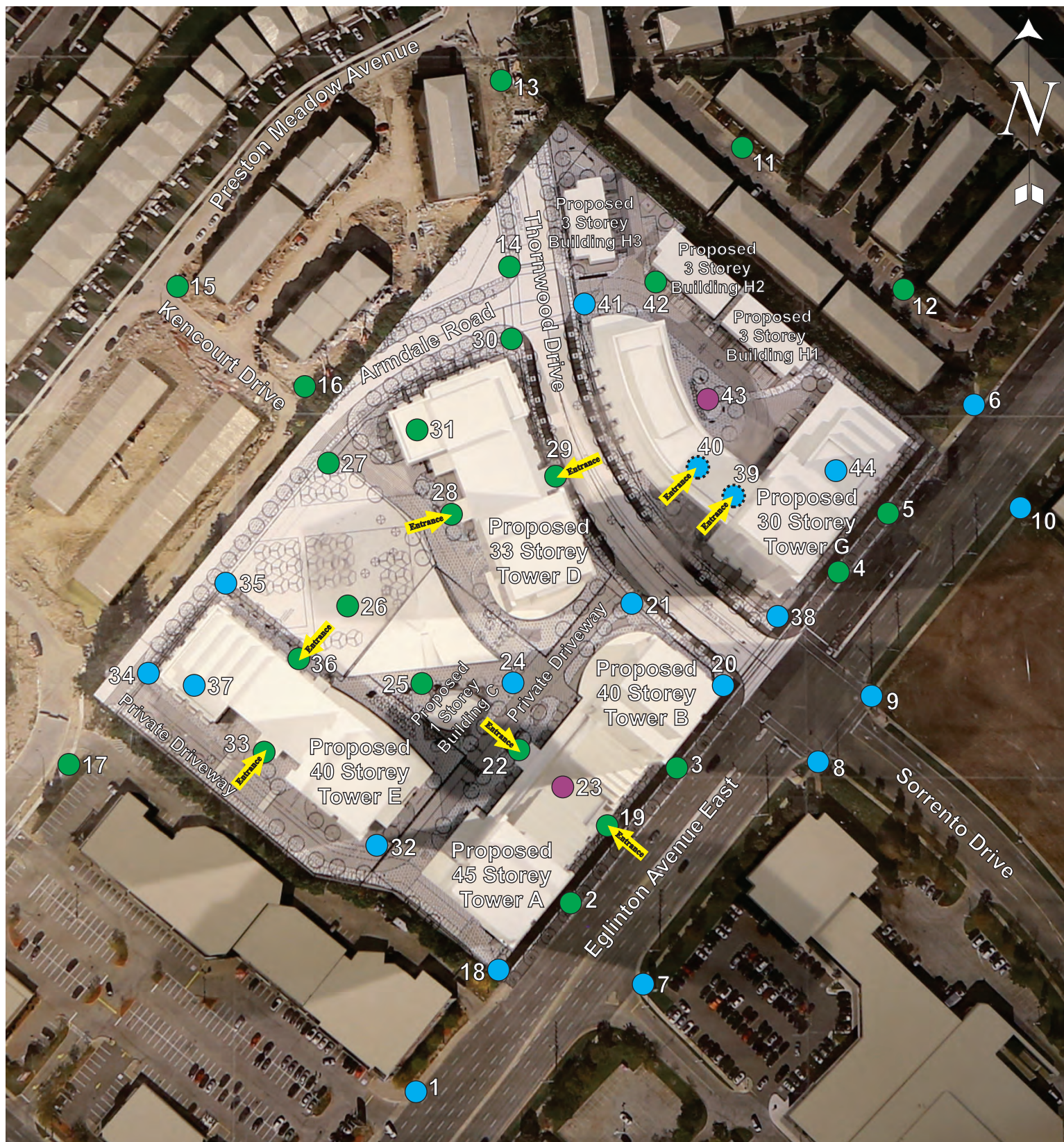
Figure 7h: Pedestrian level wind velocity comfort categories.
