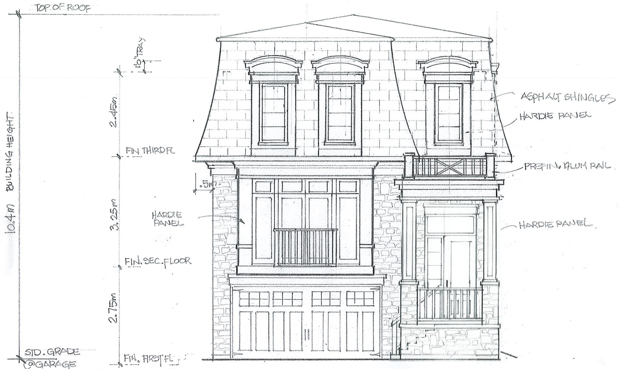
FRONT ELEVATION 8.35m MODEL
