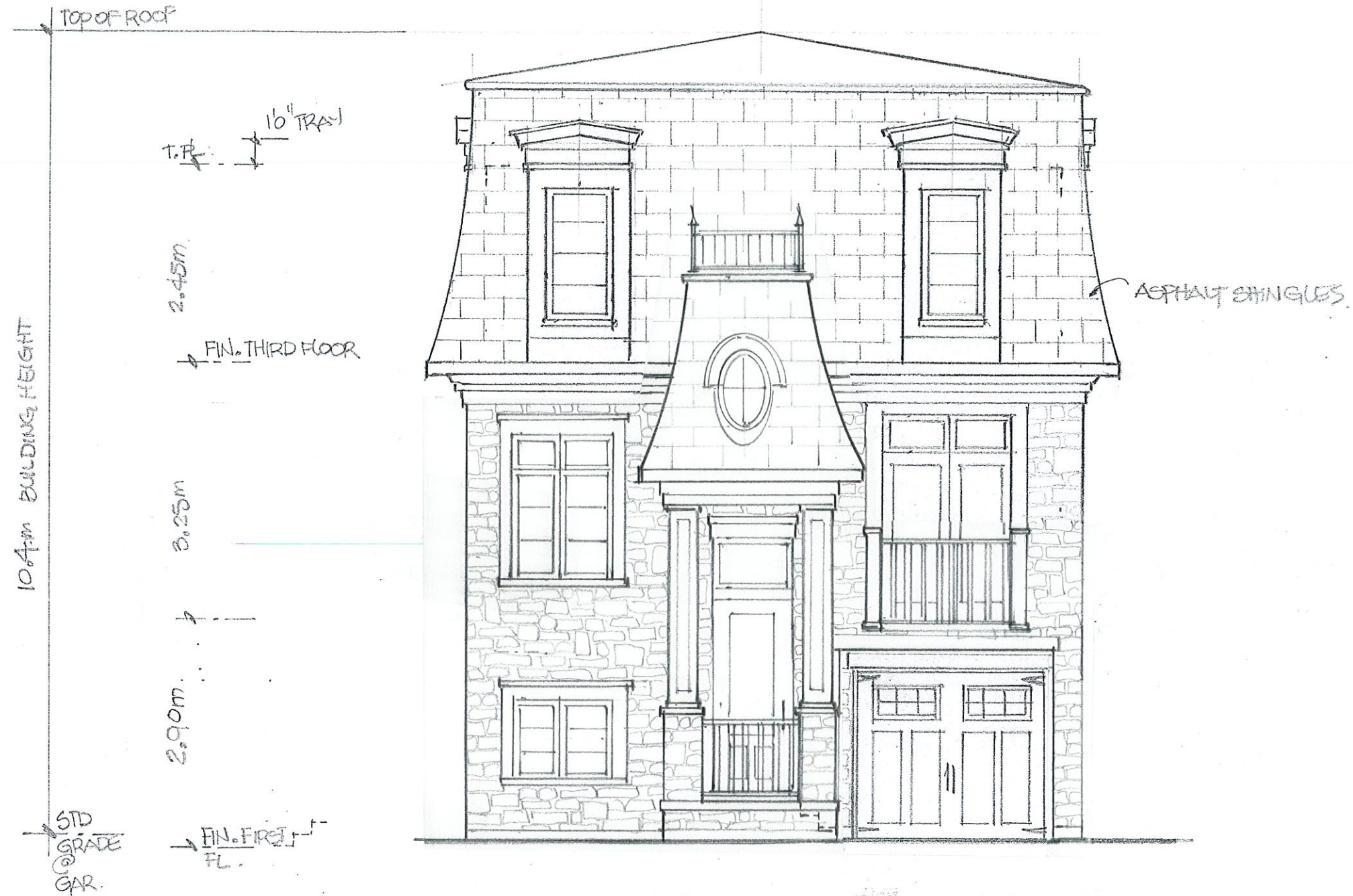
FRONT ELEVATION 7.75m MODEL
