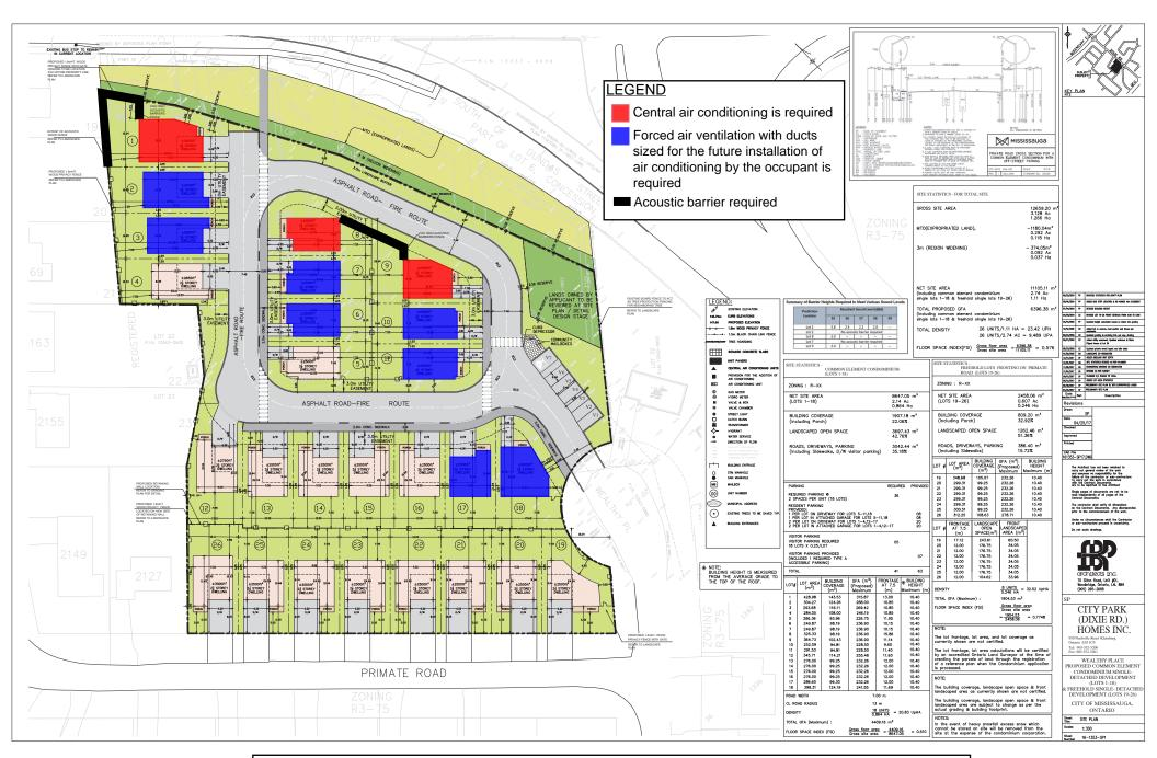
Figure B - Proposed Site Plan Showing Barrier and Ventilation Requirements
