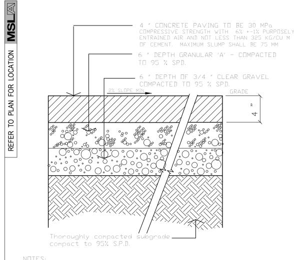
CONCRETE TO BE 30 MPa COMPRESSIVE STRENGTH WITH 6% +-1% PURPOSELY ENTRAINED AIR AND NOT LESS THAN 325 KG/CU M OF CEMENT. MAXIMUM SLUMP SHALL BE 75 MM 2. IMMEDIATELY AFTER FINISHING WITH WOODEN FLOAT, ALL WALKS, CURBS, AND WALLS SHALL
