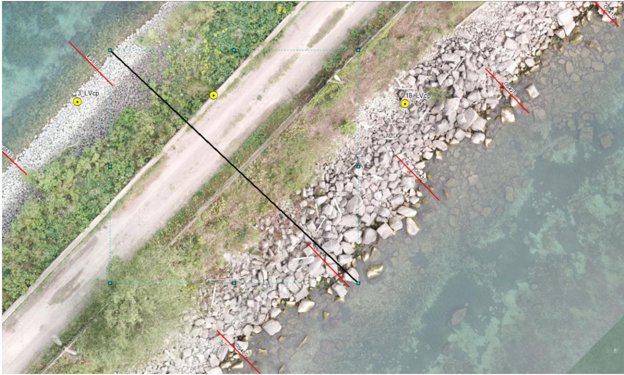
Figure 2.12: Example of high-resolution image of shoreline from processed UAV survey (red lines mark shoreline sector stations; yellow circle with black dot centre is ground control point; black line indicates section location)
