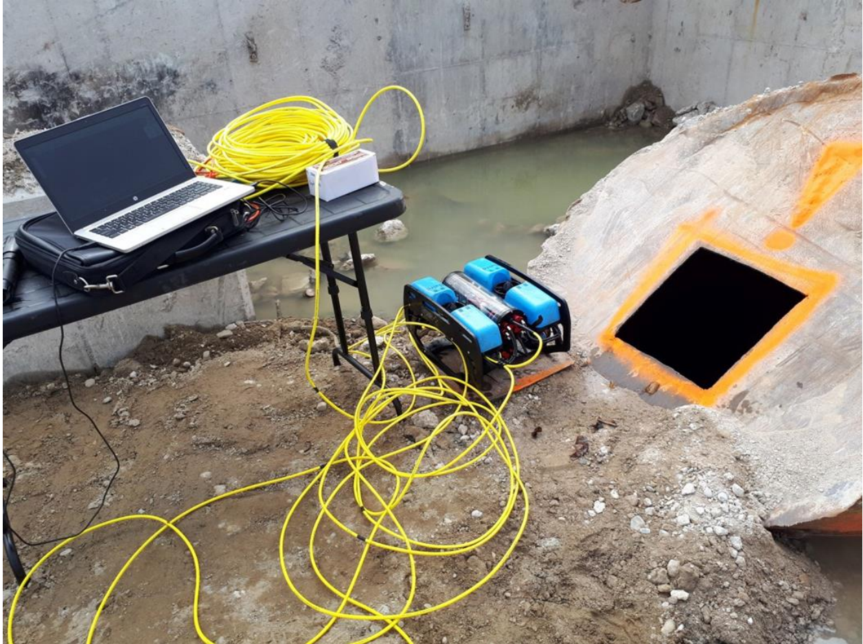
Figure 2.21: Baird submersible ROV used for underwater investigation
