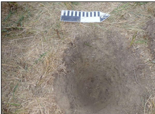
Plate 5: Typical disturbed test pit comprising dark grey clay loam laid topsoil, over brown clay fill, over subsoil.
