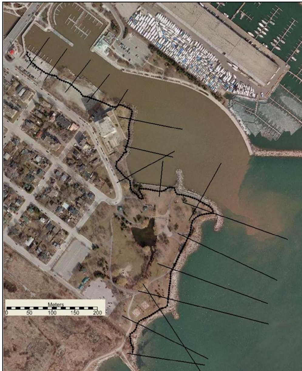
Figure 15: Location of Typical Profiles and Calculated Wave Uprush Limit
