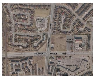
Figure 4-5: Grid roads gave way to circuitous road patterns and culde-sacs to discourage traffic from cutting through neighbourhoods; tall noise walls were erected along major streets to shield neighbourhoods from traffic noise.
