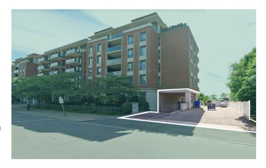
Figure 71: Loading should be located underground, internal to the building or to the rear of the buildings.
