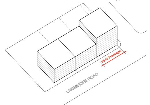
**Figure 37:** A minimum of 90% of the building shall front onto Lakeshore Road East and West and be within 0.0 m to 3.0 m.
