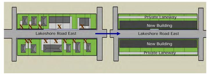
Figure C13 — Example of access consolidation which is required to make an urban street pedestrian oriented and safe.
