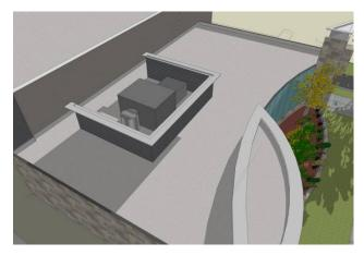
Figure 21: Provide architectural screening around roof-mounted mechanical equipment to minimize the visual impact from the street.
