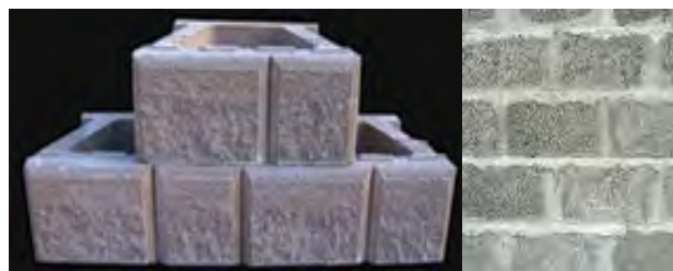
Figure B92 — Architectural concrete block is highly discouraged as an exterior building material
