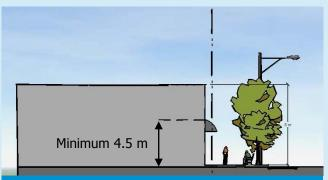
**Figure B31** — Minimum building height of 2 storeys will be permitted
