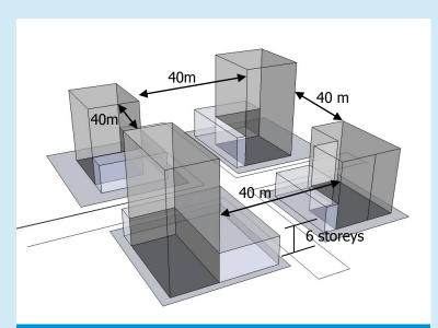
**Figure B44** — Block to block separation distance
