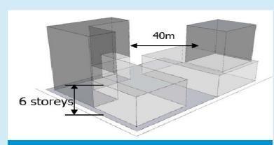
Figure B45 — Within a block separation distance
