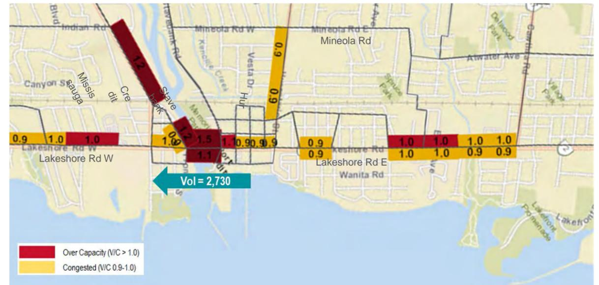
**Exhibit 3-11 Capacity Deficiencies without New Credit River Crossing (2041 BAU PM Peak Hour)**
