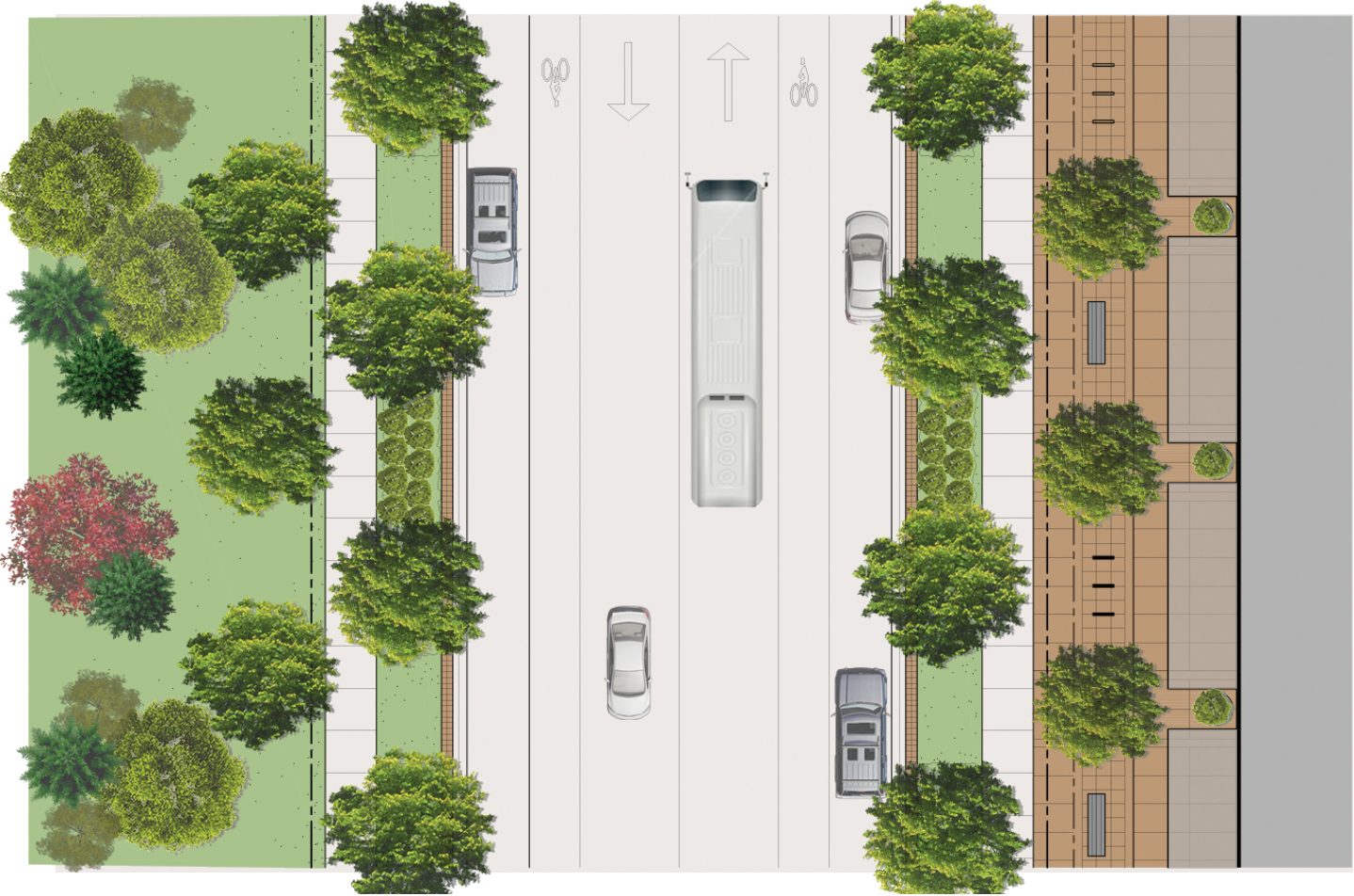
Figure 5.9.3a - Example of a bioswale integrated within an urban street right-of-way.
