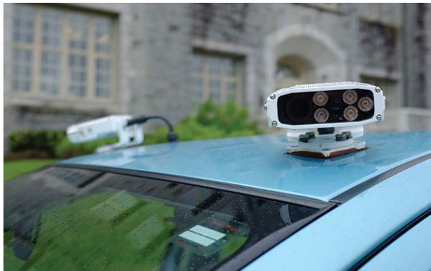
Digital Chalking using Licence Plate Recognition Technology
