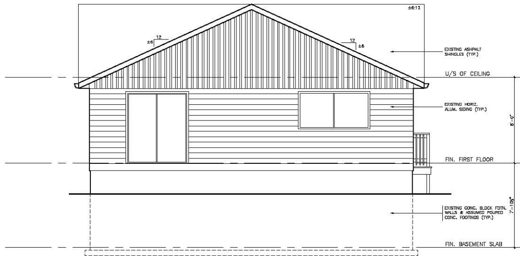
1 EXISTING REAR ELEVATION A4 1/4" = 1'-0"
