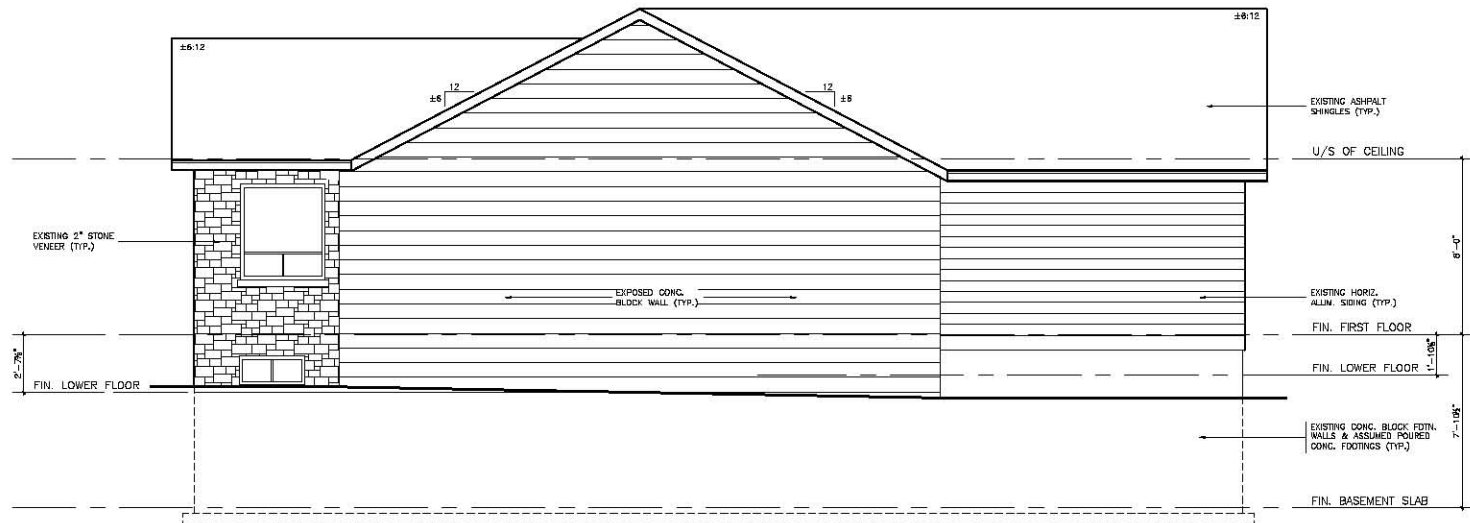
2 EXISTING RIGHT SIDE ELEVATION A3 1/4" = 1'-0"
