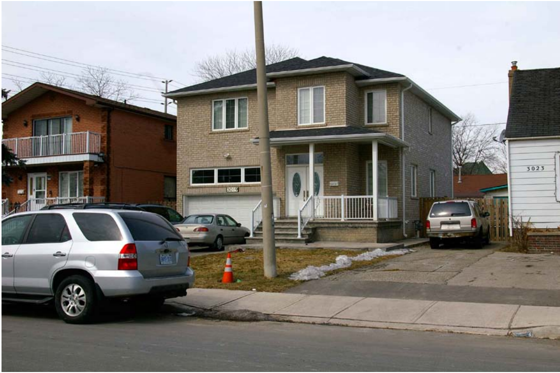
Photo 4: A two-storey replacement dwelling built in 2009 at 3019 Churchill Avenue, which features a single-door double garage with a transom window, hipped roof, raised porch and brick veneer cladding.
