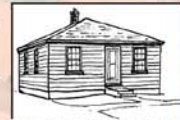
The Housing Enterprises of Canada (HEC) development includes four different styles of HEC houses. This example is a single detached, one-storey, separate dwelling with a central chimney, front entrance and a central brick chimney. In general, HEC houses have big roofs, large or no porches, concrete and concrete block with, concrete dwelling and full basements.
