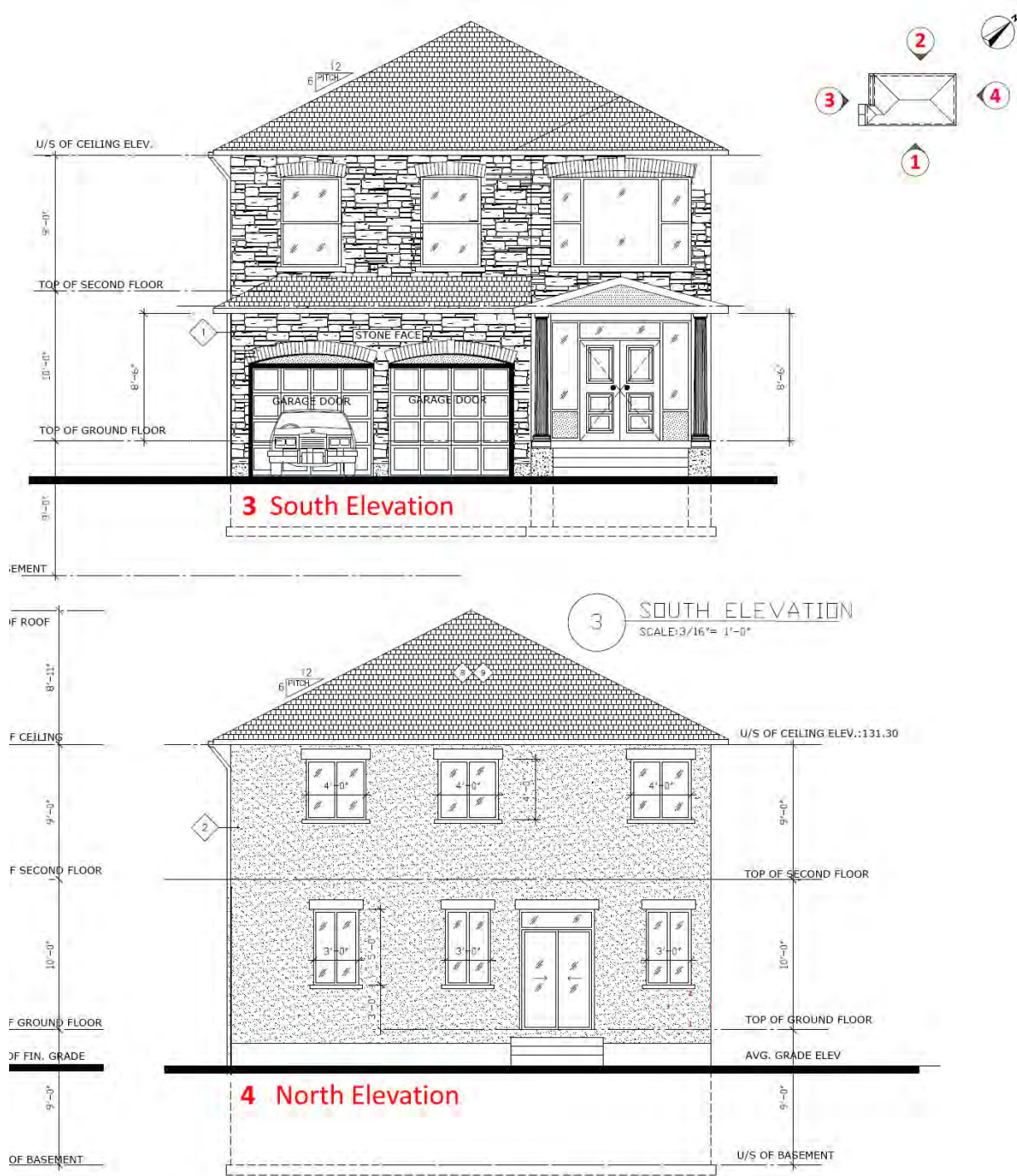
Figure 28: Front and rear elevations showing changes made by Sanpro Engineering Inc. to the front facade of the proposed dwelling based on alterations proposed in Figure 27 .
