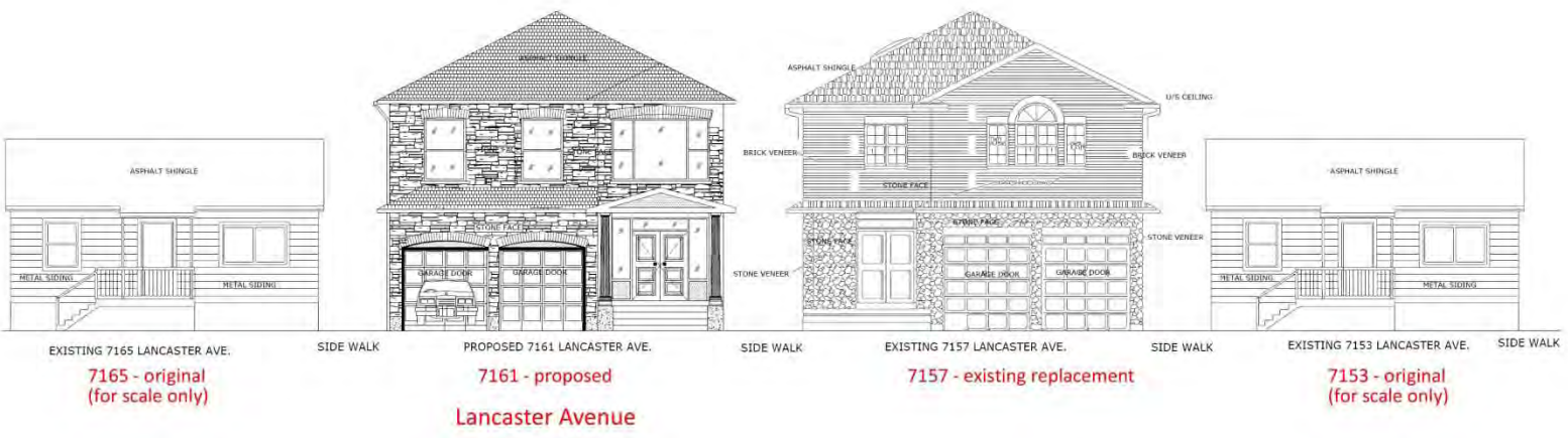
Figure 30: Streetscape elevation showing the proposed two-storey dwelling at #7161, the existing replacement dwelling of similar size at #7157 and the two original bungalows on either side.
