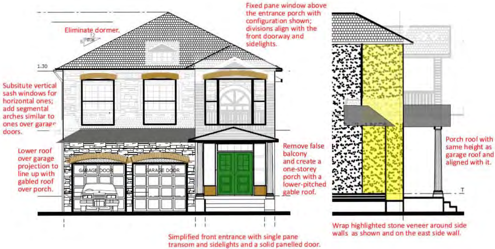
Figure 27: Overlay of front facade and part of one side elevation showing alterations recommended and illustrated by the author of this report.
