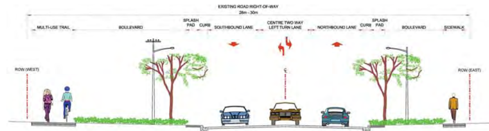
Typical Cross-Sections Under Consideration THREE LANE SECTION
