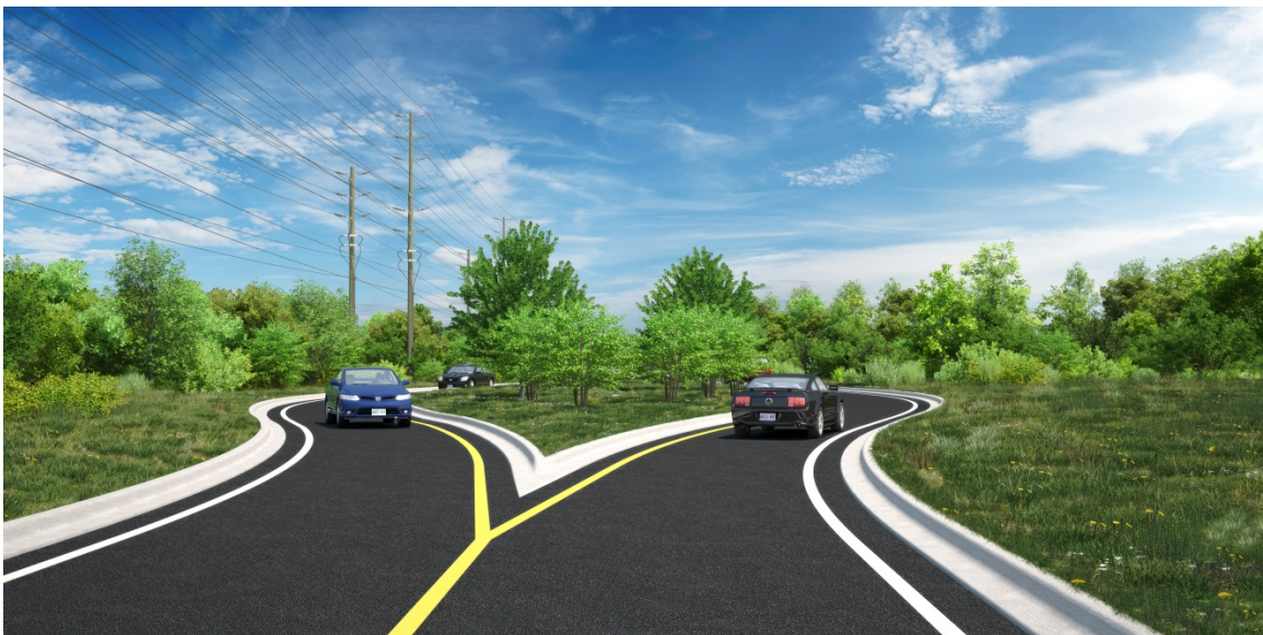
View Looking East along Sheridan Park Drive extension corridor showing potential median (horizontal deflection)
