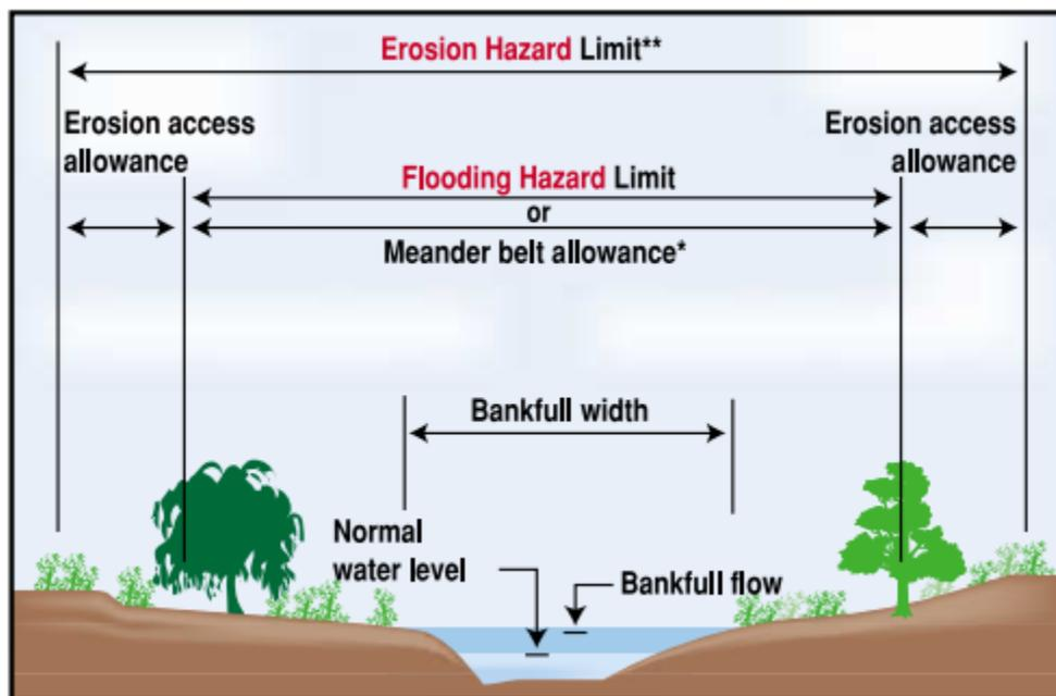
Figure 3-6. MNRF Guideline for Determining an Erosion Hazard Corridor within Unconfined Systems Such as Applewood Creek.
