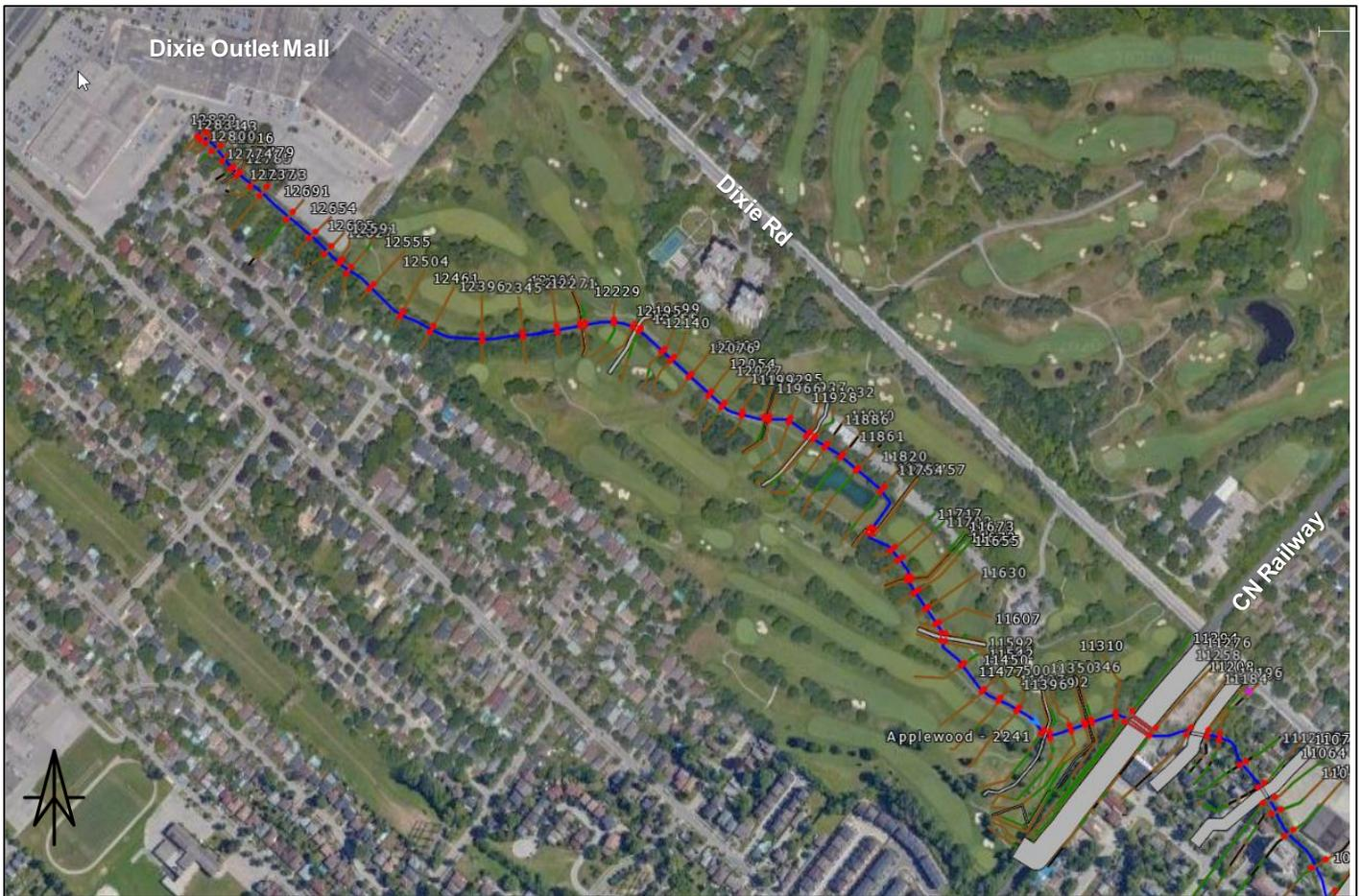
Figure 3-7. Existing HEC-RAS Schematic of Applewood Creek within the Study Area.
