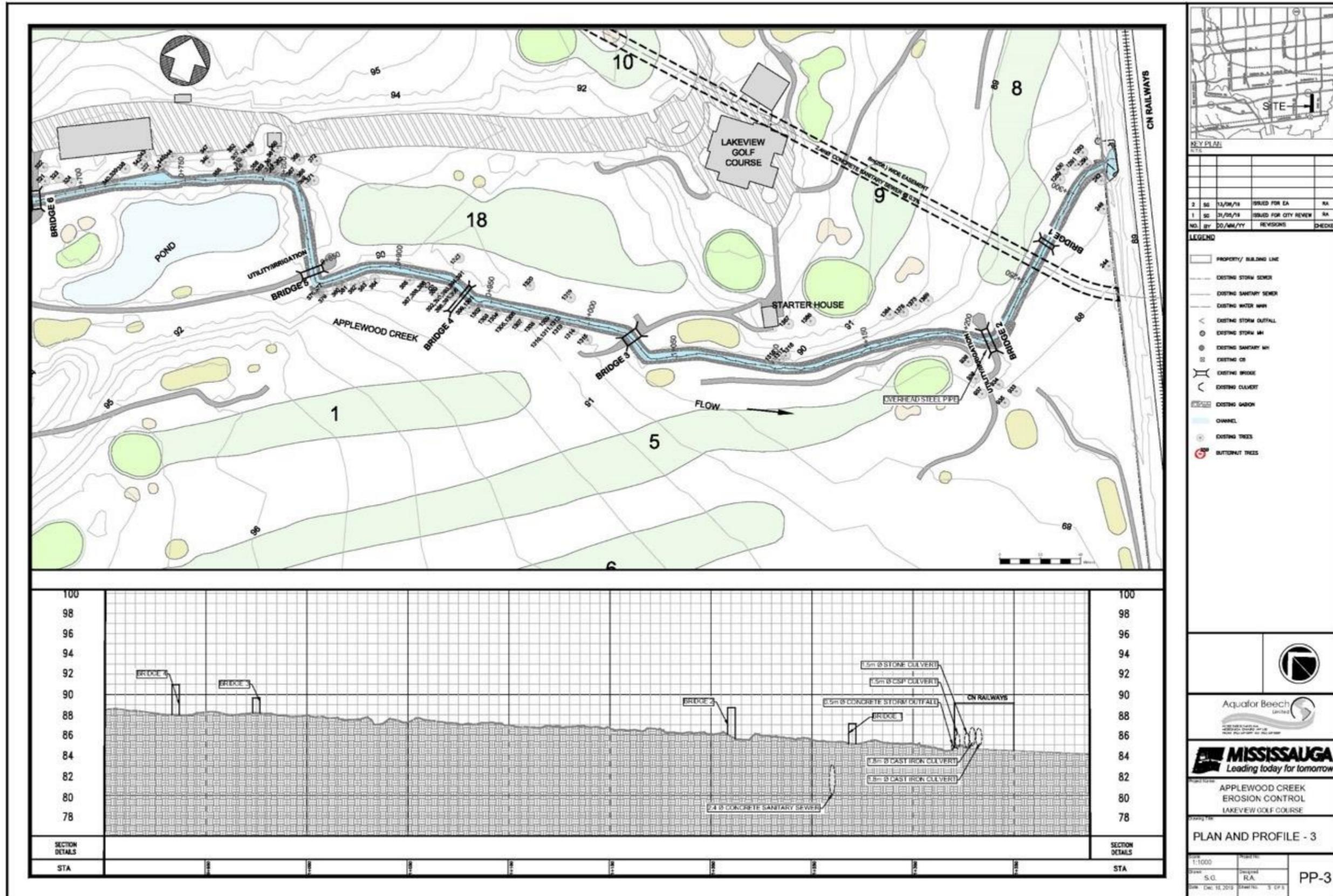
Figure 3-3. Topographic Survey Presented as Plan and Profile of Applewood Creek (3 of 3).
