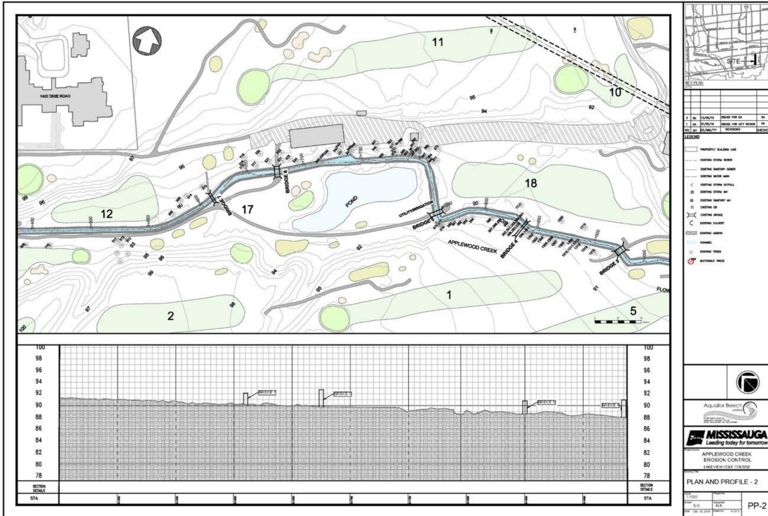
Figure 3-2. Topographic Survey Presented as Plan and Profile of Applewood Creek (2 of 3).
