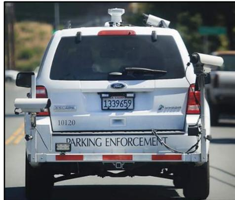
A computer logs the plate number, the GPS location of the vehicle, the date, and the time. The system can use the internet to link with PBLP and mobility payment (pay by cell) systems and check the validity of monthly parking permits (as license plates act as parking permits).
