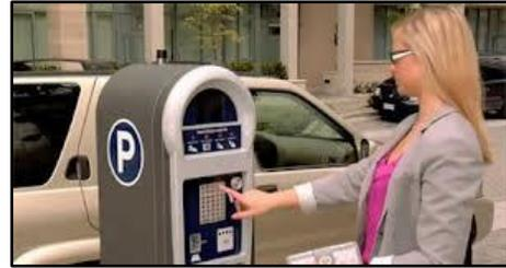
PBLP uses solar power and a cellular network. The system processes credit card transactions in real-time and stores the statistical/financial information recorded on a cloud server.
