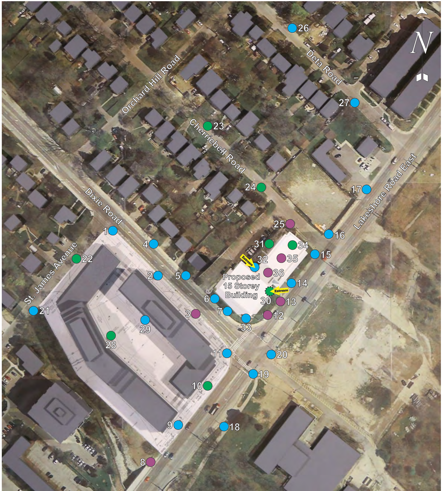
Figure 7j: Pedestrian level wind velocity comfort categories.
