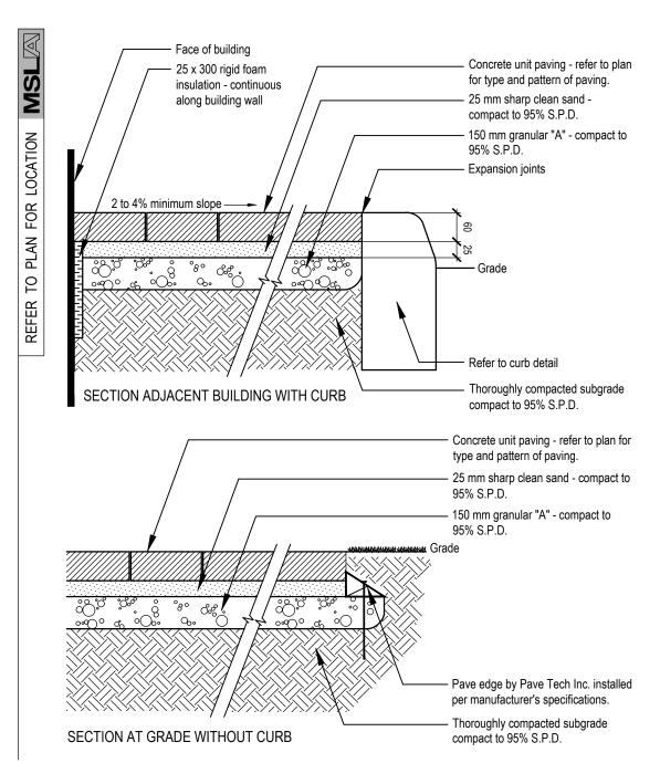
PRECAST CONCRETE PAVER INSTALLATION DETAIL
