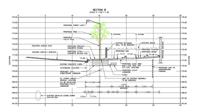
LEXISTING HYDRO CABLE ALONG EGLINTON AVENUE EAST TO BE RELOCATED INTO PROPOSED UTILITY CORRIDOR AS PER DETAILED DESIGN BY ALECTRA (IN PROGRESS)
