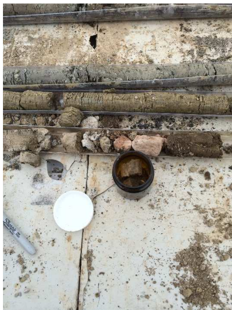
Photograph 7 Red brick debris found in BH5 at around 1' bgs.
