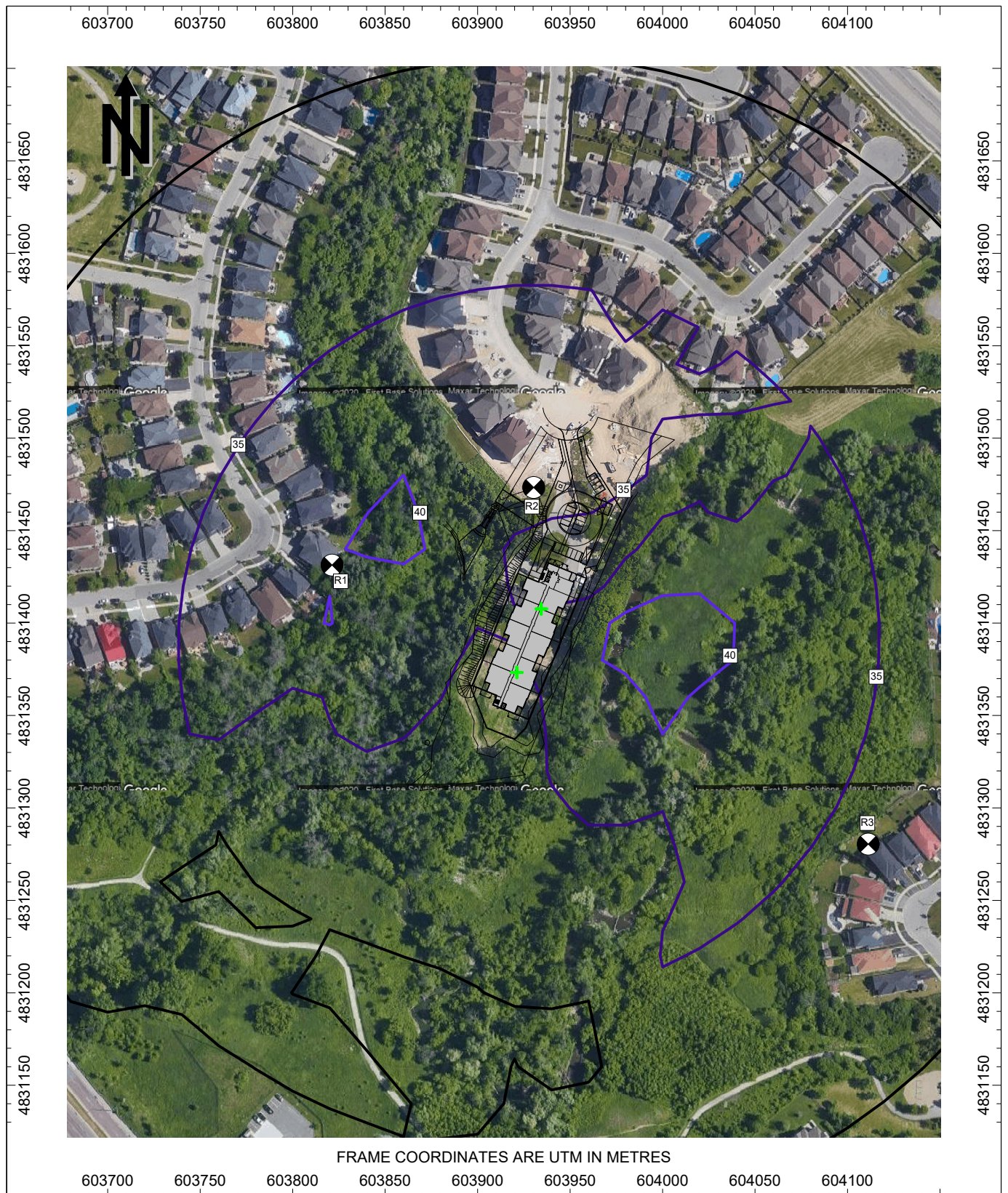
Figure 4: Predicted Stationary Source Sound Level Contours, Leq1hr [dBA]
