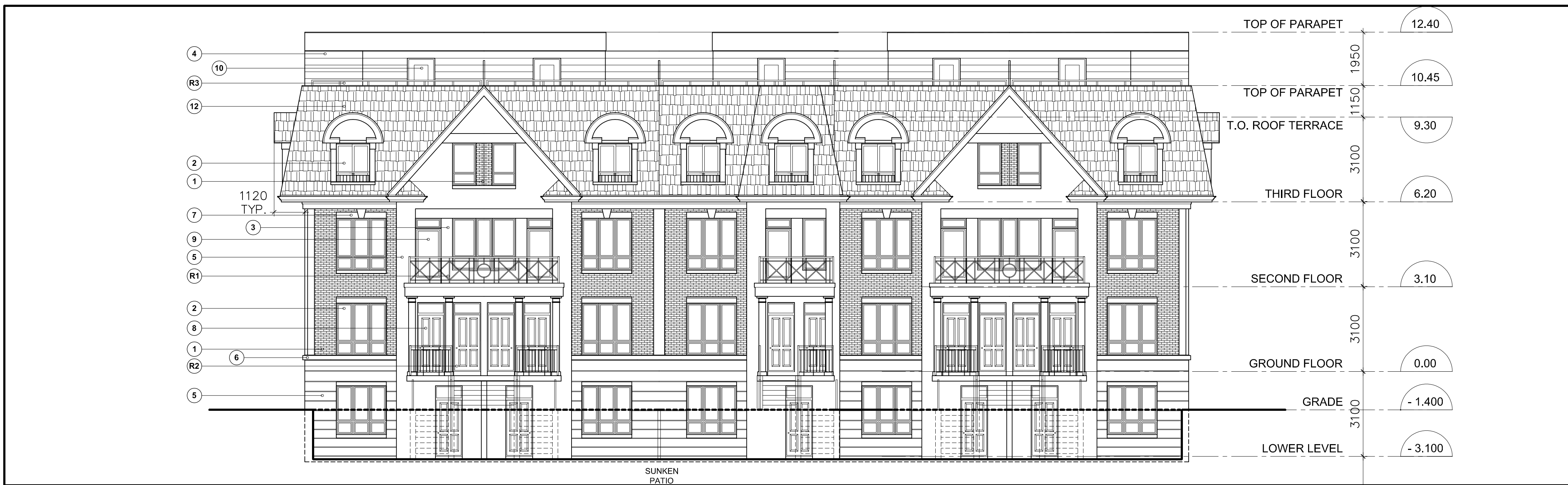
Building E&F - North Elevation 2 1:100 RZ-07
