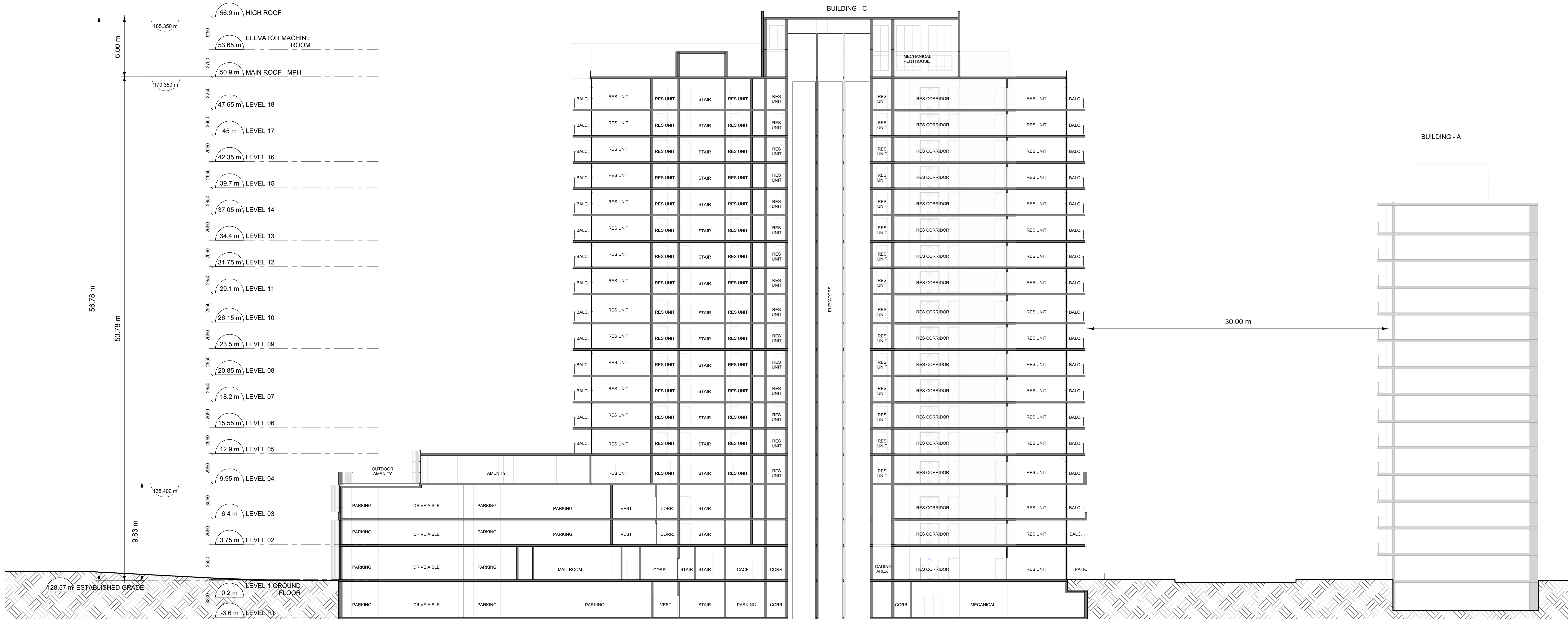
2 NORTH-SOUTH BUILDING - C SECTION A-302 / Scale: 1 : 150
