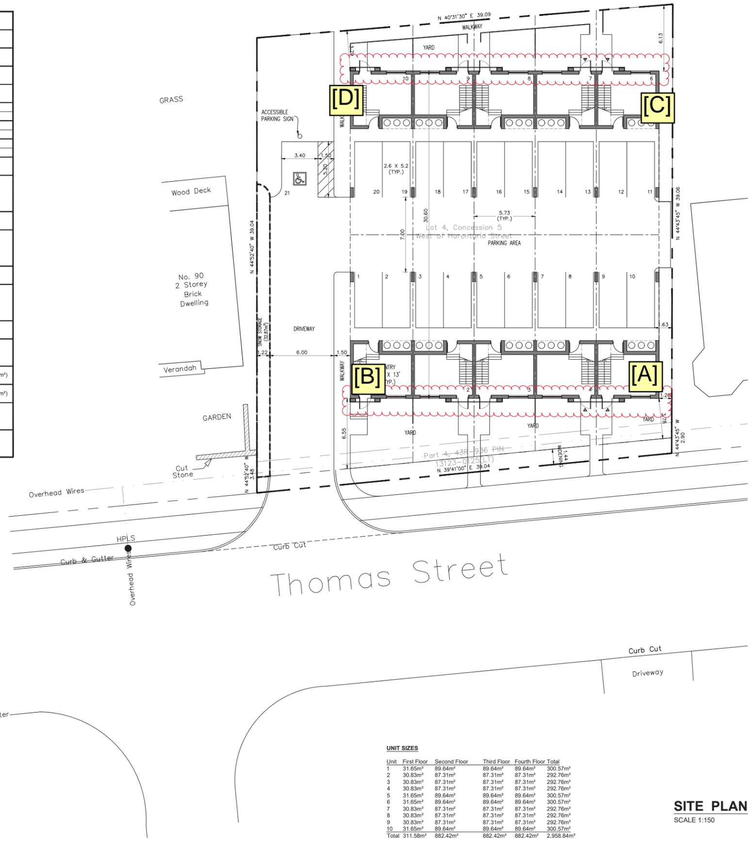
**Figure 2: Proposed Site Plan Showing Prediction Locations**
