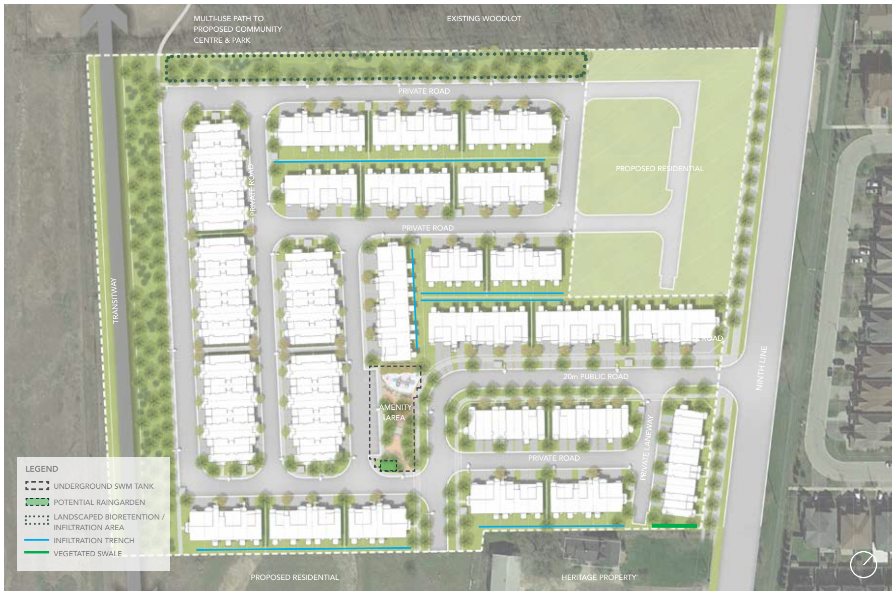
Figure 2.3 - Ninth Line South conceptual plan indicating schematic locations of storm water retention features
