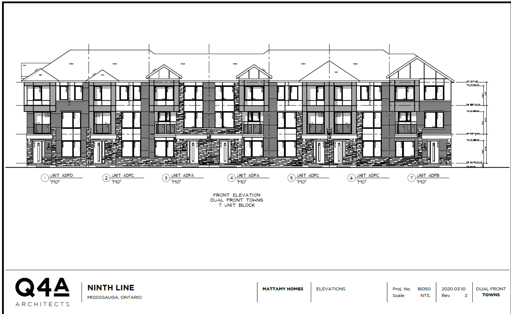
Figure 7: Dual Front Towns, 7 Unit Block – Front Elevation (Q4A Architects 2020)
