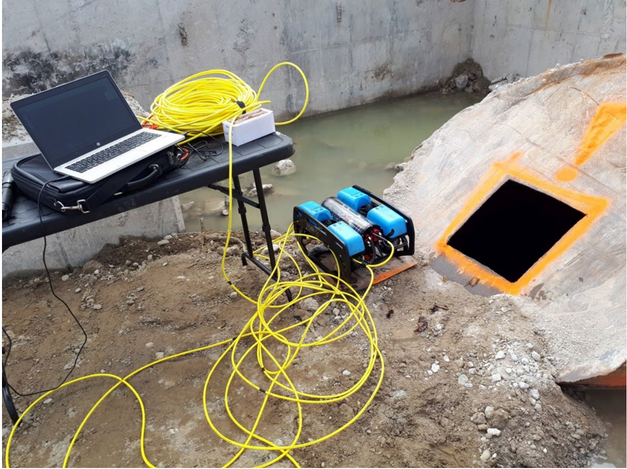
Figure 2.21: Baird submersible ROV used for underwater investigation
