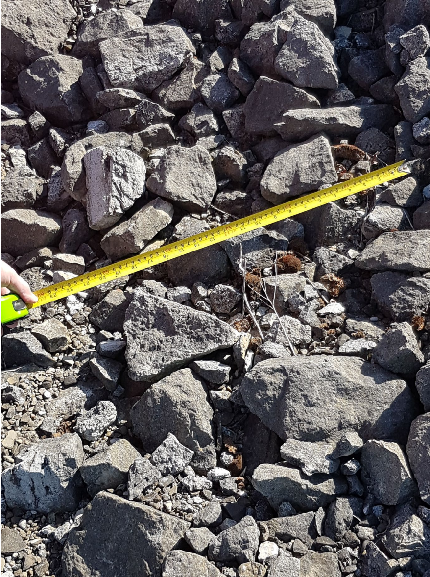
Figure 2.61: Example of riprap stone size at Intake Forebay/Channel South (IFS340)
